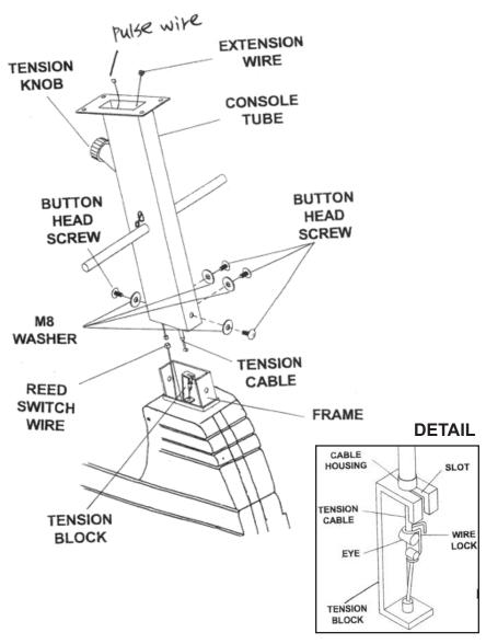
**6.** Connect EXETENSION WIRE in CONSOLE TUBE to REED SWITCH WIRE in FRAME. Connect the TENSION CABLE in CONSOLE TUBE to the TENSION BLOCK in FRAME (See Detail). Secure CONSOLE TUBE to FRAME with BUTTON HEAD SCREWS and WASHERS.
